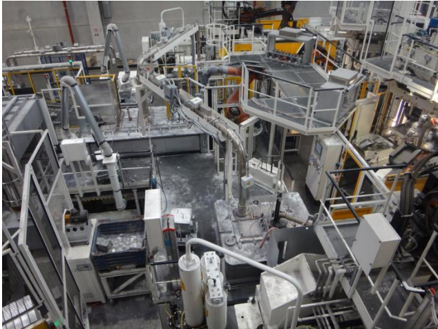
Fig.2. GGG Casting Line with a Melting Capacity of 1.400 kg Mg/h
