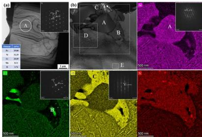
Fig.3 TEM bright-field image and SADE pattern of as-cast Fe35Ni35Cr20Mn10Ti6 HEA: (a) dendritic trunk; (b) inter-dendritic zone
