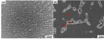
Fig.2 SEM images of as-cast Fe35Ni35Cr20Mn10Ti6 HEA
