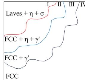
Fig. 5 The microstructure distribution diagram of as-cast Fe35Ni35Cr20Mn10Ti6 HEA.
