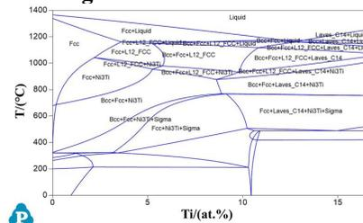
Fig.1 The pseudo-binary phase diagram of (Fe<sub>35</sub>Ni<sub>35</sub>Cr<sub>20</sub>Mn<sub>10</sub>)-Ti system, calculated by Pandat software
