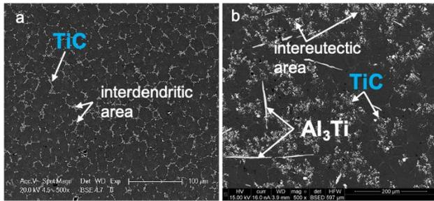
Figure 2. SEM-BSE microstructure of the Al 1000/TiC (a) and Al-7Si/TiC (b)
