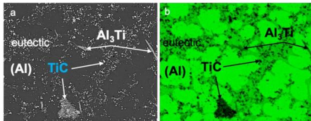
Figure 3. SEM-BSE microstructure of the Al-7Si/TiC composite (a) and corresponding SEM-EDS elements distribution map (b)
