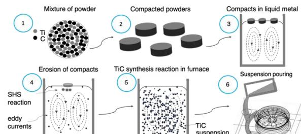
Figure 1. Schema of the in-situ TiC/Al-base composites manufacturing process
